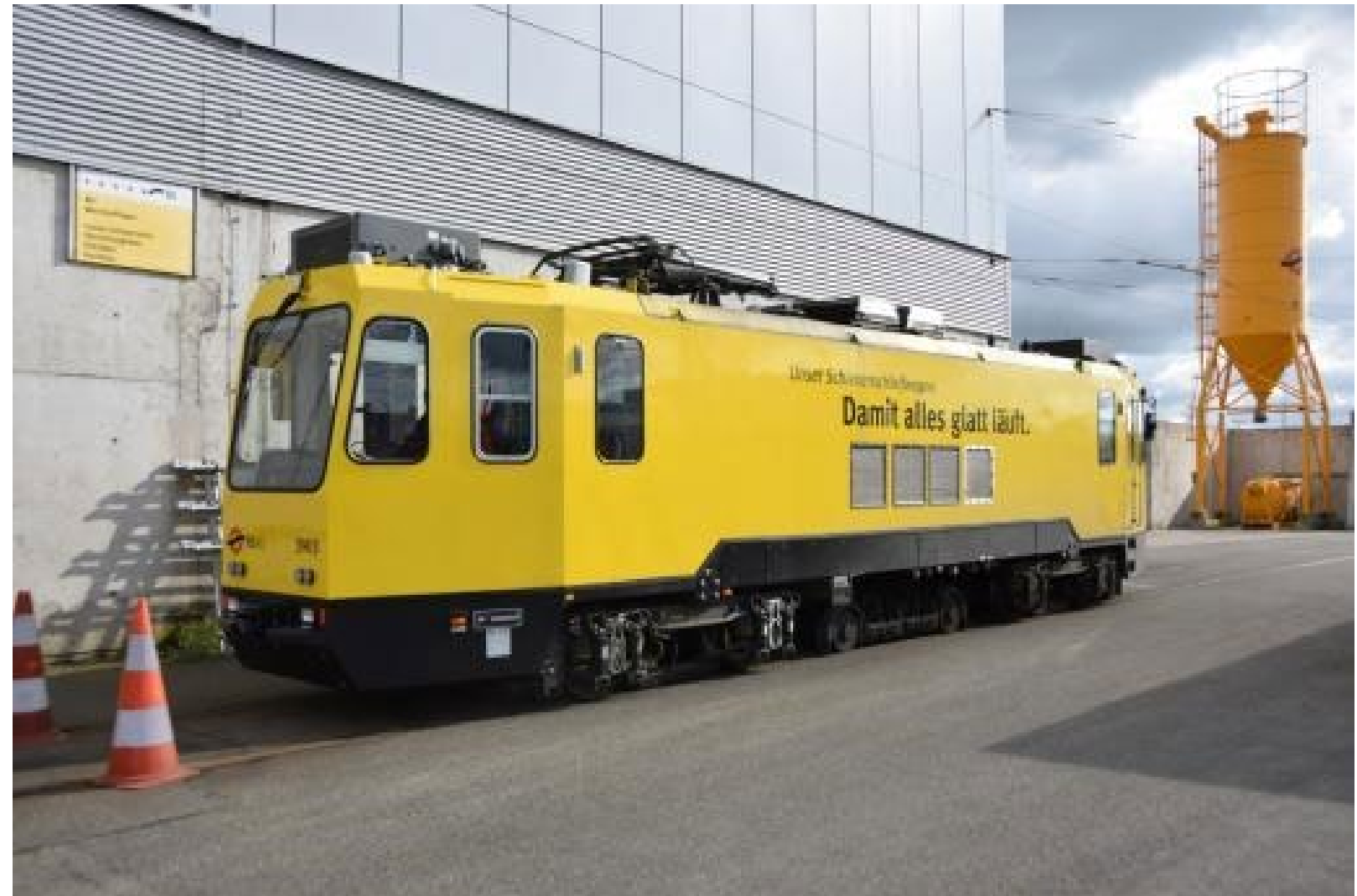
Rail grinding wagon, Bremen, Germany
